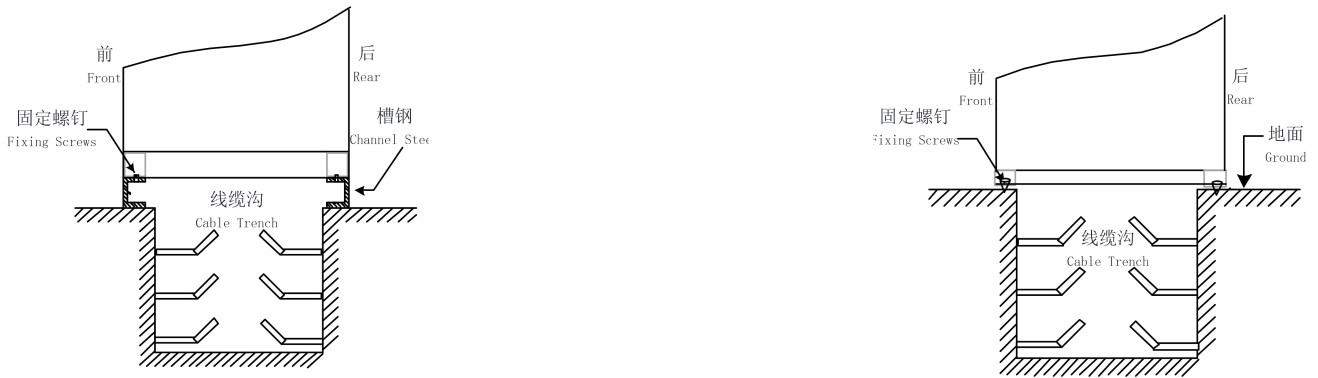
(a) Schematic diagram of the equipment fixed to the channel (b) Schematic diagram of the equipment fixed to the ground
